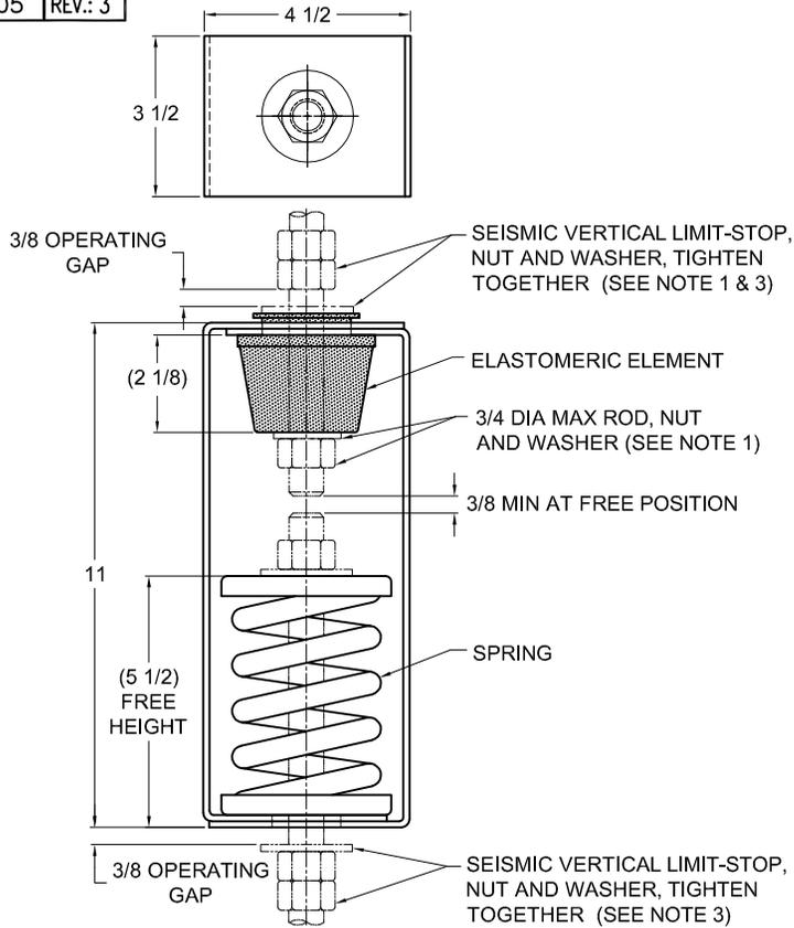
**TYPE HRS-2D PRE-COMPRESSED ELASTOMERIC & SPRING HANGERS FOR 2" NOMINAL DEFLECTION**
